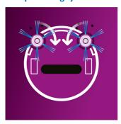
First two long brushes swipe dirt and dust into the path of the robot. Then, the nozzle picks up dirt and dust thanks to its powerful motor. Lastly, the click-on mopping pad enhances the cleaning by collecting even the finest dust from your floors.
