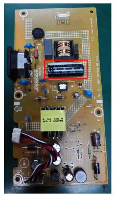
Remove electrolyte capacitors (red mark) from printed circuit boards
