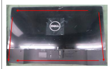
Use Penknife to separate the bezel and rear cove follow the arrows in sequence, then you can take out rear cover.
