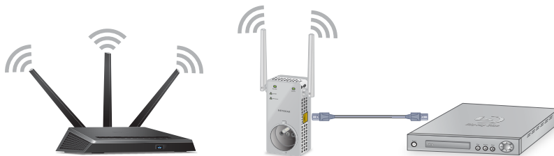
Figure 4. Connect a device to the extender's Ethernet port
