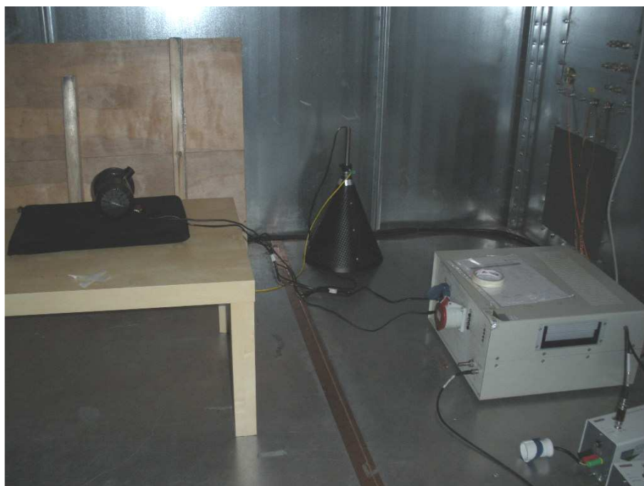
Photograph 2: Set-up for measurement of disturbance voltage
