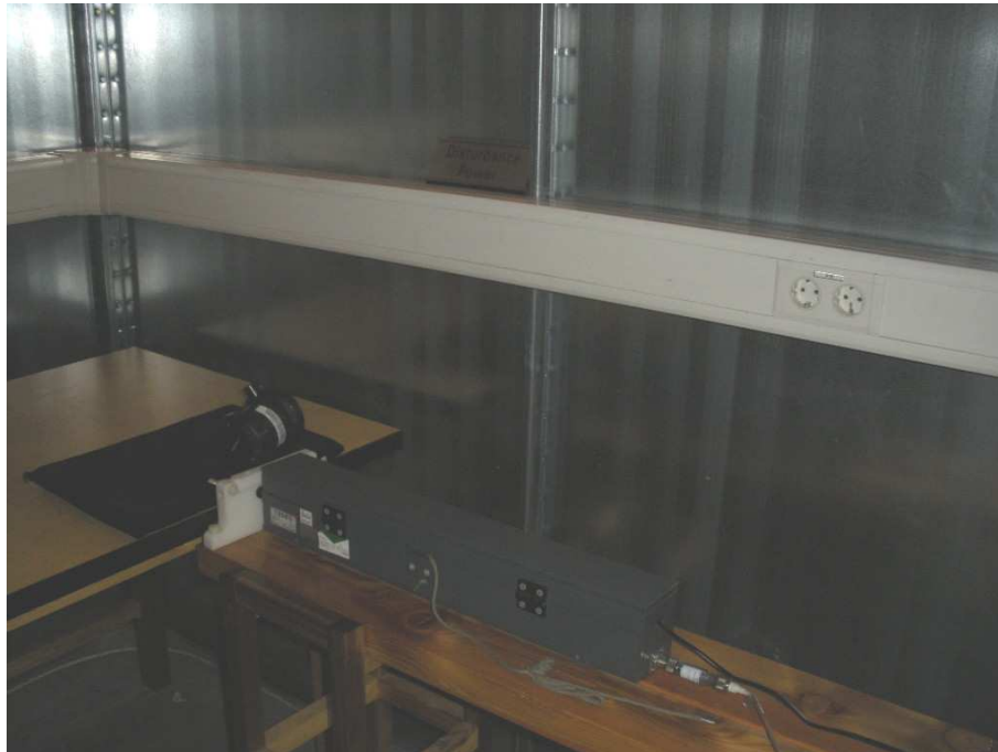
Photograph 3: Set-up for measurement of disturbance power
