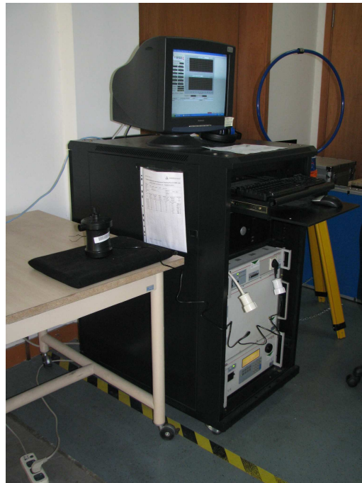
Photograph 2: Set-up for measurement of disturbance voltage
