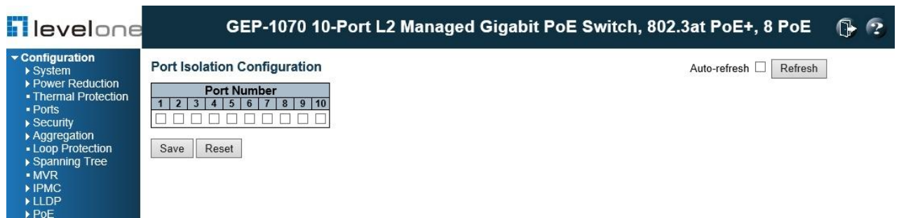
Figure 70: Port Isolation Configuration
