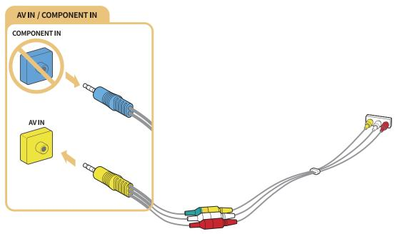
Connect AV (composite) equipment to AV In only. Do not connect to Component In.
