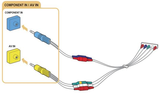
To use component equipment, connect both a component cable (blue) and an AV cable (yellow).
