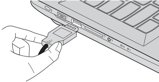
The first time you plug a USB device into a particular USB port on your computer, Windows automatically installs a driver for that device. After the driver has been installed, you can disconnect and reconnect the device without performing any additional steps.
