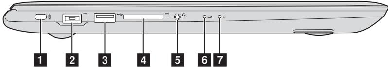
**1 Kensington slot** Attach a security lock (not supplied) here to help protect your computer from theft and unauthorized use. You can attach a security lock to your computer to help prevent it from being removed without your permission. For details on installing the security lock, please refer to the instructions shipped with the security lock that you have purchased.
