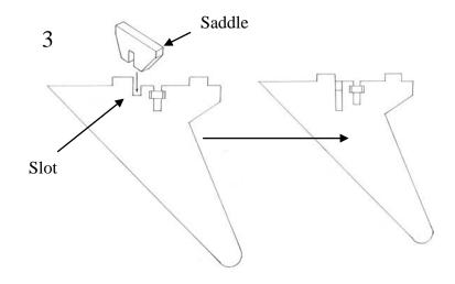
Slide the Saddle into the slot in the 2 Legs
