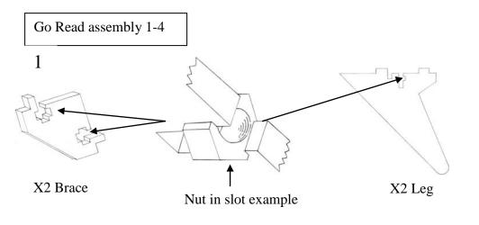
Slide the 6 nuts into the slots in the Brace and Legs. If tight, simple slide in from the opposite side of the component.
