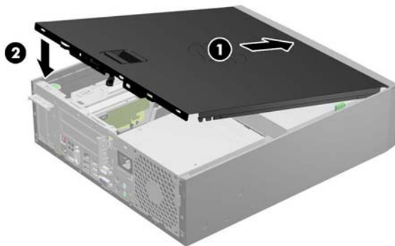
Figure 2-2 Replacing the Computer Access Panel
