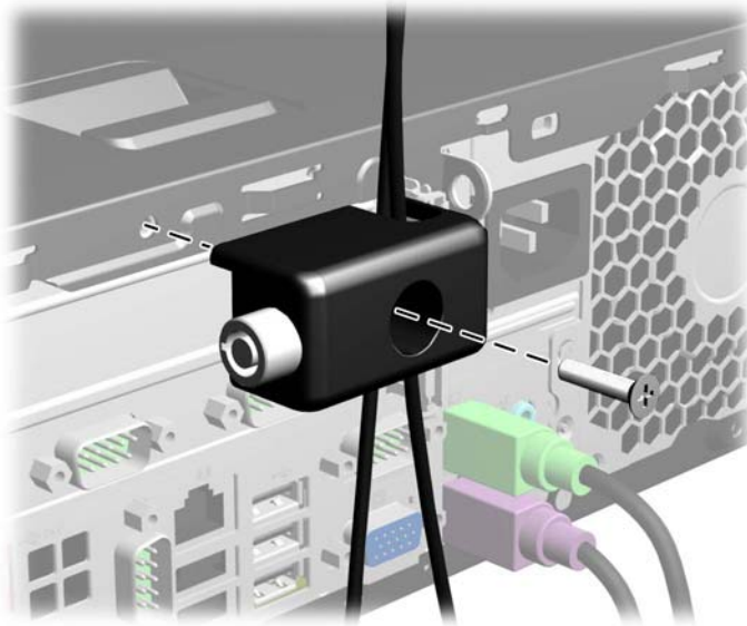
Figure A-8 Attaching the Lock to the Chassis
