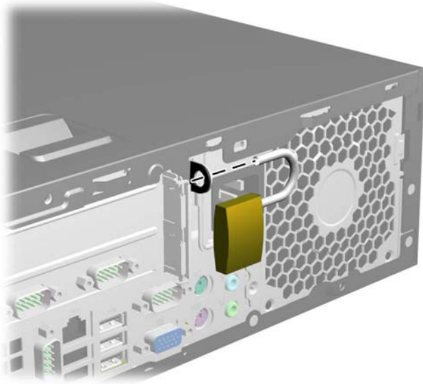
Figure A-2 Installing a Padlock
