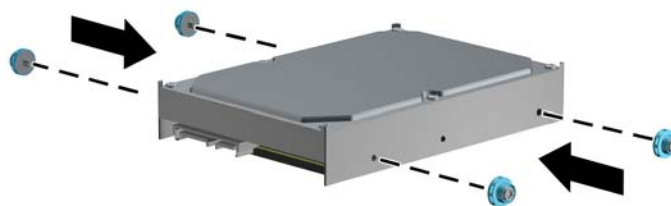
Figure 2-66 Installing Primary Hard Drive Guide Screws
