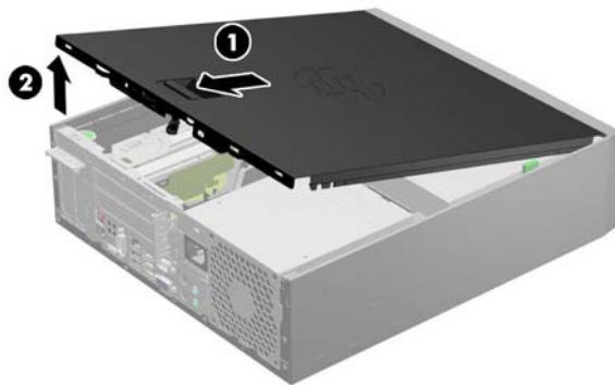
Figure 2-1 Removing the Computer Access Panel
