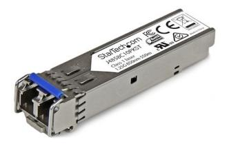
The J4859C10PKST is a ten-pack of our HPE J4859C compatible fiber transceiver module that has been designed, programmed and tested to work with HPE brand switches and routers. It delivers dependable 1 GbE connectivity over fiber cable, for 1000BASE-LX compliant networks, with a maximum distance of up to 10 km (6.2 mi).
