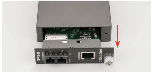
**Step 2:** Unscrew and remove the bay cover of any of the empty slots in the chassis.
