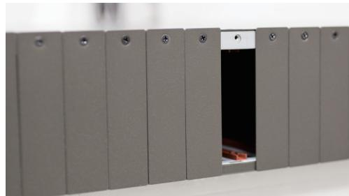
**Step 3:** Place the media converter board into the vacant chassis slot and secure it using the thumb screw on the converter's front panel.
