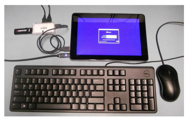
After making the necessary connections and powering on the tablet, as soon as the Dell splash screen is displayed, press the F12 on the keyboard or hold the Volume-Up button to bring up the one-time boot selection menu.
