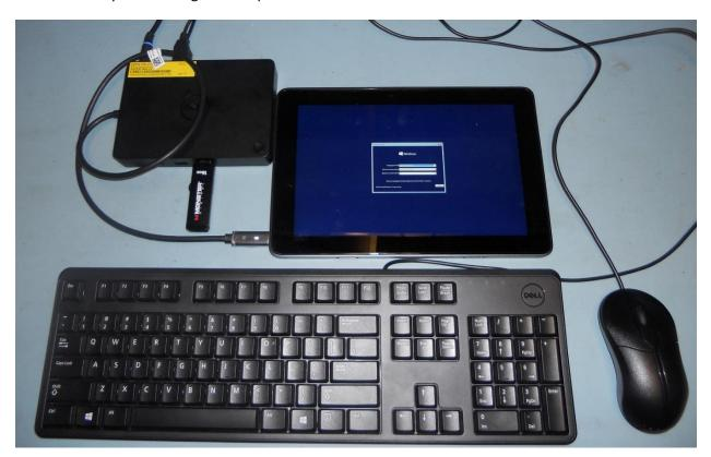
With the Venue Pro 5056, if a USB-C docking unit is not available, another method possible is to use a USB-C charging adapter with a USB3.0 or 2.0 hub on the system's external USB port to provide connection for the keyboard, mouse and USB flash installer.
