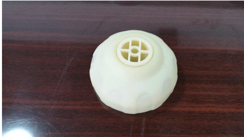
Fig. 4 – Jet model F4081 (smaller), Measured Opening Area is 0.000373 m 2 .
