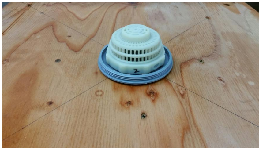
Fig. 2 - Suction Outlet Model F4078, Measured Opening Area is 0.0027228 m 2 .
