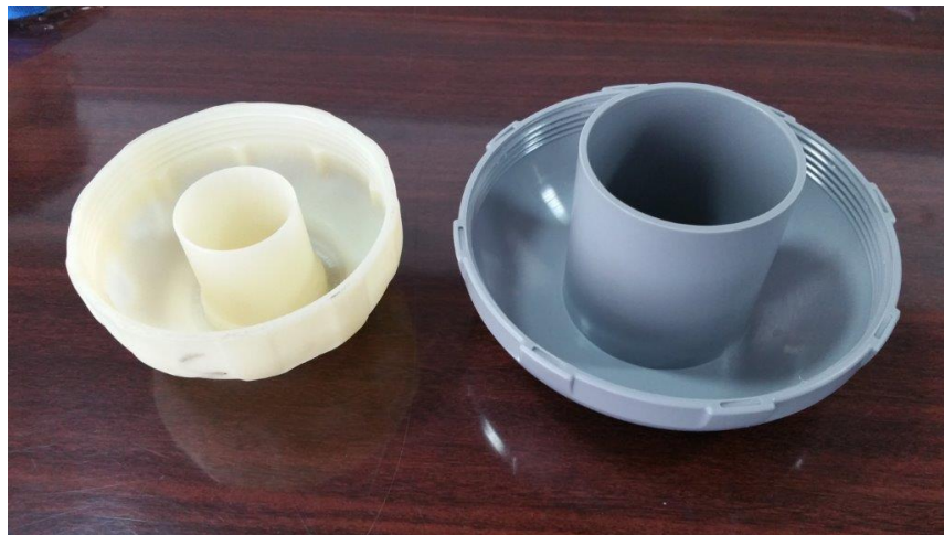
Fig. 3 – Jet model F4080 (larger); Measured Opening Area is 0.001024 m 2 .
