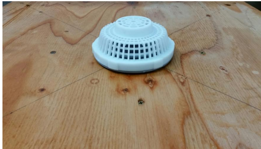
Fig. 1 - Suction Outlet Model F4077, Measured Opening Area is 0.00461944 m 2 .
