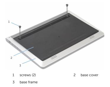
**3** Using a plastic scribe, pry the base cover off the base frame.
