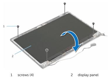
Disconnect the display cable from the display panel.
