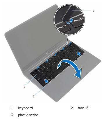
Carefully turn the keyboard over and place it on the palm-rest assembly.
