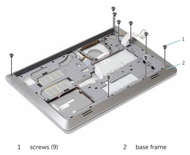
5 Using your fingertips, starting from the rear, pry the base frame off the palm-rest assembly.
