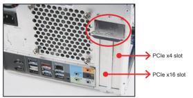
Install the PCIe x4 / PCIe x16 card into the PCIe x4 / PCIe x16 slots
