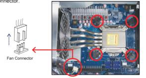
3. Remove the ICE module from the chassis and put it aside.
