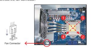
11. Fasten the Smart Fan to the chassis with the four thumbscrews.
