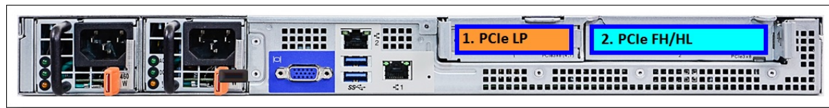
Figure 7. PCIe slot locations
