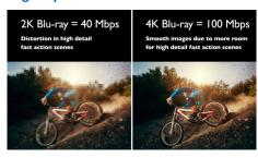
4K Blu-ray format supports more than twice the peak bitrate of 2K Blu-ray which comes in especially handy when watching action movies which have fast paced scenes with a lot of detail. The 100 Mbps peak bitrate of 4K Blu-ray provides enough headroom to store the extra data required to encode high detail fast action scenes and avoid block artifacts.
