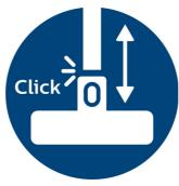
The ActiveLock couplings allow you to easily connect and disconnect the different nozzles
