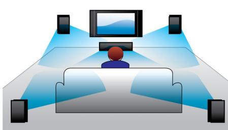
A built-in Dolby Digital decoder eliminates the need for an external decoder by processing all six channels of audio information to provide a surround sound experience and an
