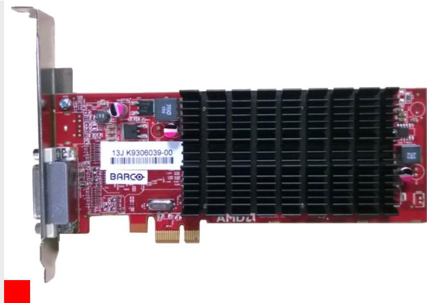
The MXRT-1451 is a low-profile and small form factor PCIe display controller used to drive HIS, RIS and patient list monitors up to 1920 x 1200 display resolution. Since it's a PCIe x1 card, it fits in workstations where all PCIe x16 slots are occupied.
