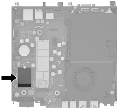
7. Disconnect both antenna cables from the WLAN module.
