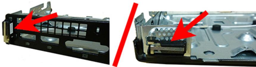
16. Remove the front transceiver from the inside of the computer by pressing the tab to disengage the transceiver and removing the transceiver (arrow in following image points to the tabs on the inside of the computer).
