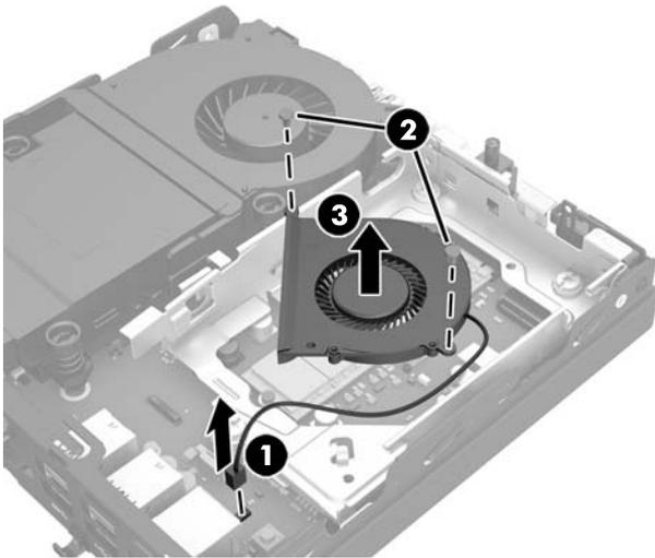
To install the secondary fan, reverse the removal procedure.
