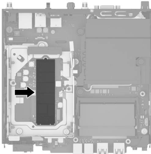
7. Remove the screw securing the SSD to the system board.
