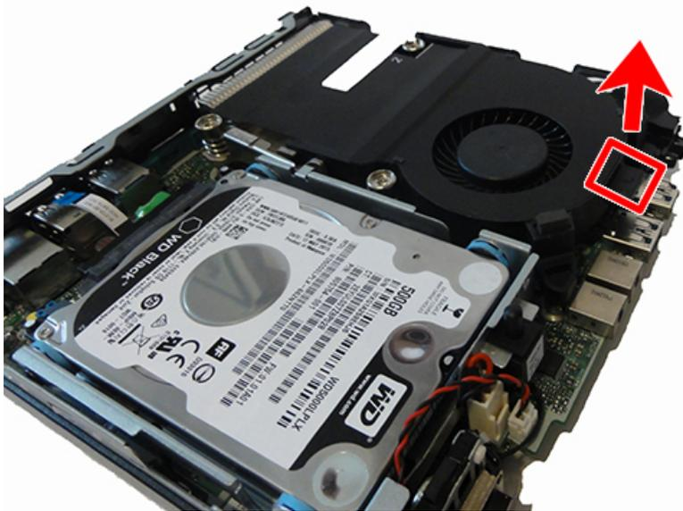
4. Disconnect the fan plug from the system board, and then lift the fan out of the chassis.
