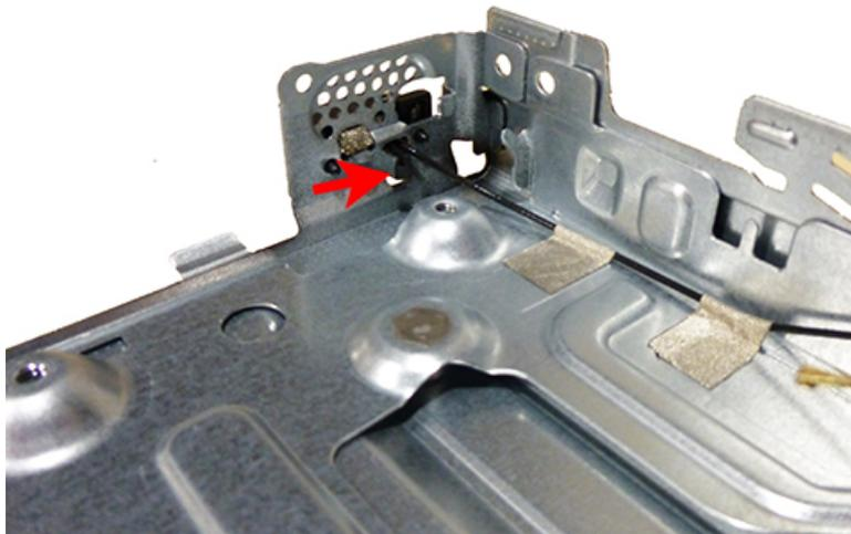
17. Remove the rear transceiver from the inside of the computer by pressing the tab to disengage the transceiver and removing the transceiver (arrow in following image points to the tabs on the inside of the computer).
