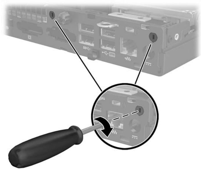
10. Feed the external antenna cable through each hole and screw the antenna into position.
