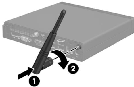
11. Connect the external antenna cables to the WLAN module.
