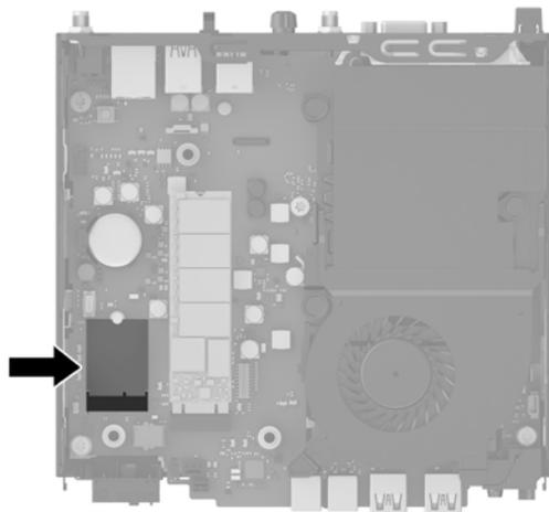
7. Disconnect the internal antennae from the WLAN module.
