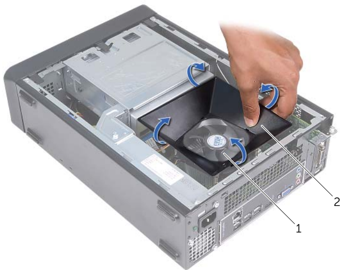
1 processor fan and heat-sink assembly 2 fan shroud
