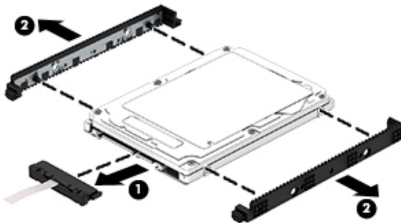
Reverse these procedures to reassemble and install the hard drive.
