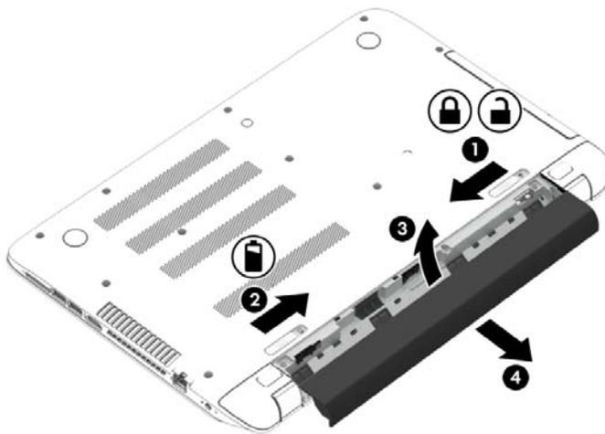
Reverse this procedure to install the battery.
