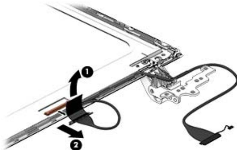
12. If it is necessary to replace the webcam/microphone perform the following: Lift the module (1) from the adhesive holding it in place on the display bezel and disconnect the module connector (2) if you have not already done so when removing the display cable.
