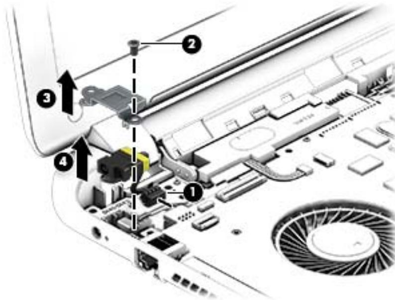
Reverse this procedure to install the power connector cable and bracket.
