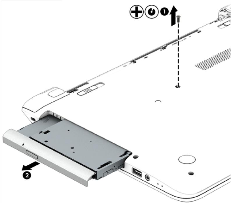
3. Remove the optical drive from the computer.
