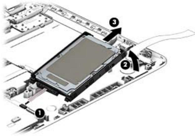
If it is necessary to disassemble the hard drive:
