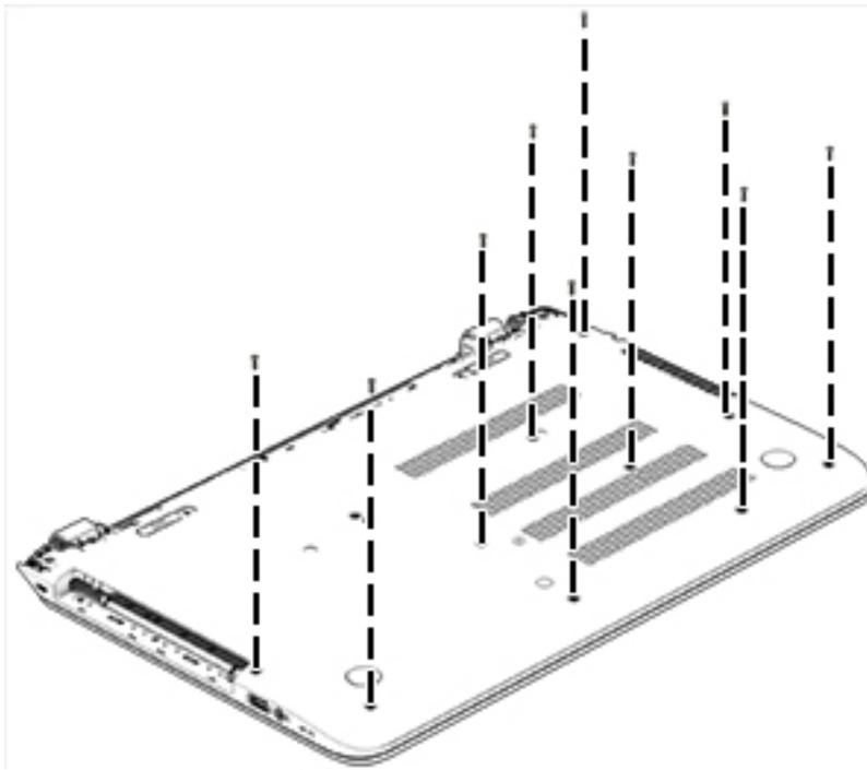
3. Remove five screws (1) around the battery area, three broadhead screws (2) in the optical drive bay and one screw (3) near the display hinge.
