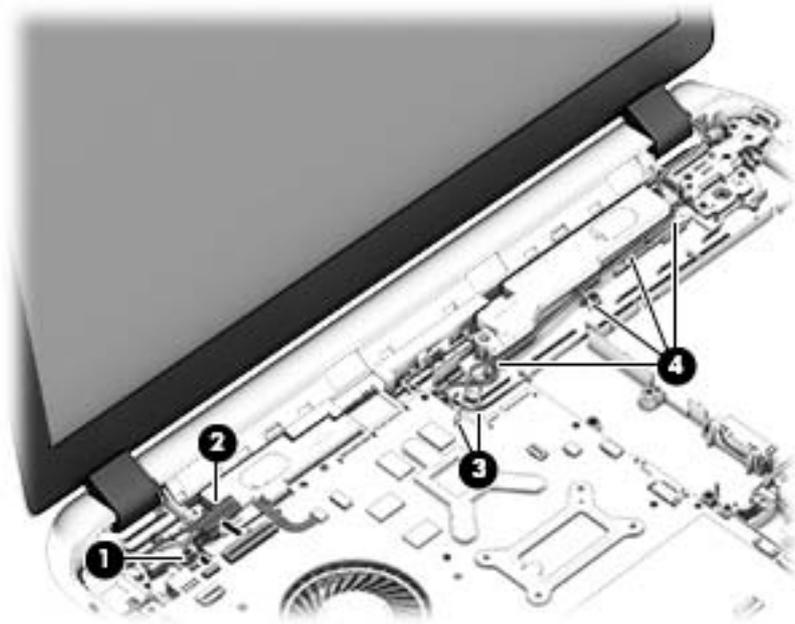
4. Remove the power connector cover by removing the Phillips screw (1) and lifting the cover (2).
