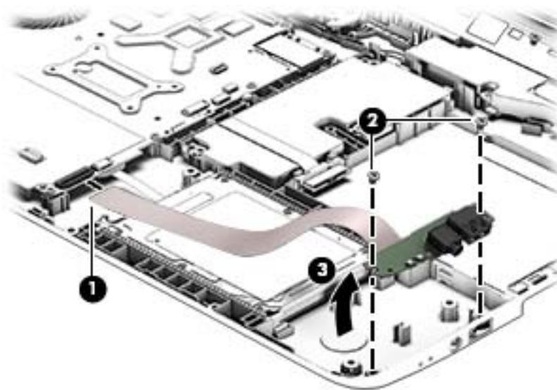
Reverse this procedure to install the USB board and cables.
