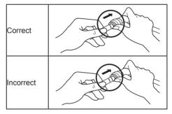
If the end of the water supply line is damaged, it should be trimmed to ensure it does not leak when refitted.
