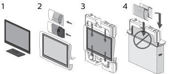
To avoid damage to the screen, do not pack the stand on the same side as the TV screen, refer to the step 4 above.
