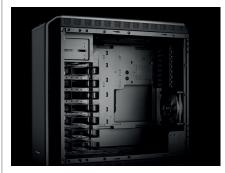
**MB-tray:** The motherboard tray can be repositioned vertically, to suit individual space requirements, or installed alongside the left panel with redefined airflow. It is removable for use as a bench table.
