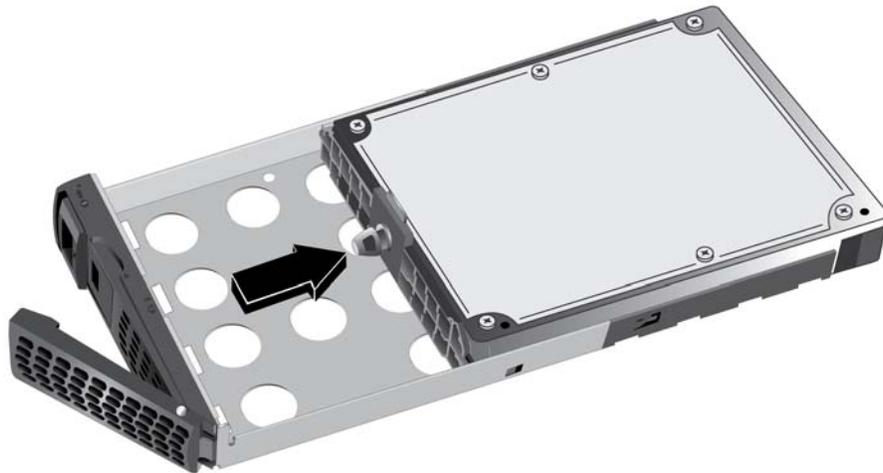
6. Remove the old HDD from the mounting bracket.
