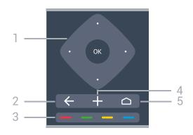
1 - OK key / Arrow / navigation keys To confirm a selection or setting. To navigate up, down, left or right.
