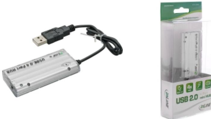
The Mini USB Hub has 4 USB Type A ports for connecting up to 4 USB 2.0 / 1.1 or 1.0 devices. This hub is bus powered, it requires no external power supply. The connected USB devices together should not require more than 500mA, or have their own power supply. The Pocket Mini USB Hub has an integrated USB 2.0 cable.
