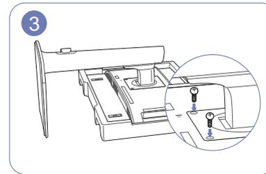
Fasten the screws to tightly fix the stand.
