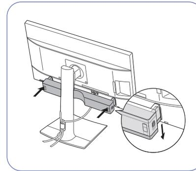
Insert the connector bars of the sound bar into the slots on the sides, then push down in the direction of the arrow to secure the sound bar in place.
