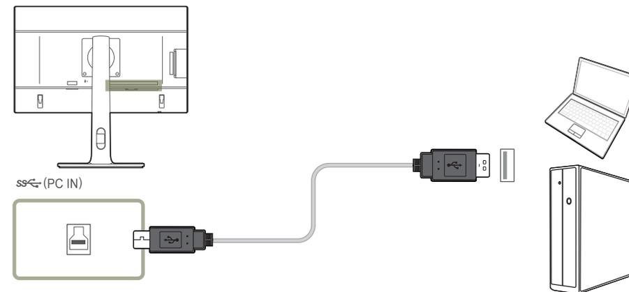
Connect the USB cable to
