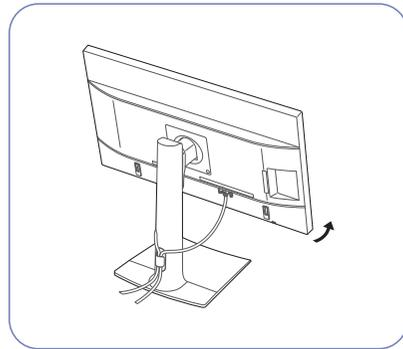
Tilt the product with all the cables connected, as shown in the picture.
