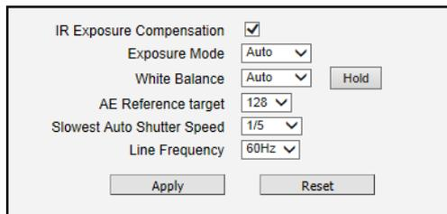
The screenshot shows the 'IR Exposure Compensation' settings menu. The 'IR Exposure Compensation' checkbox is checked. Below it are several settings: 'Exposure Mode' set to 'Auto', 'White Balance' set to 'Auto' with a 'Hold' button to its right, 'AE Reference target' set to '128', 'Slowest Auto Shutter Speed' set to '1/5', and 'Line Frequency' set to '60Hz'. At the bottom are 'Apply' and 'Reset' buttons.
