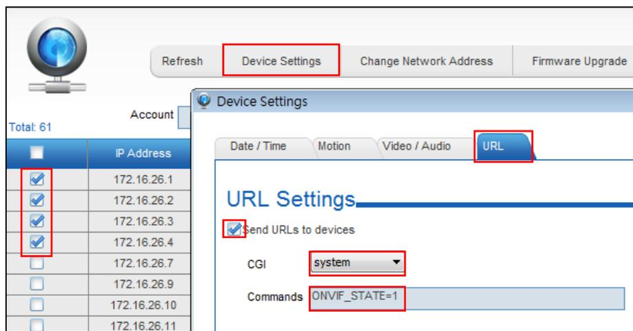
The IP Utility interface shows a table of devices and a "Device Settings" panel. The "URL" tab is selected in the settings panel.
