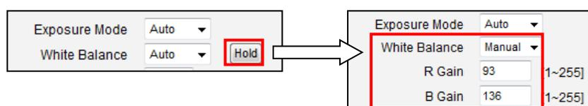
For advanced users, there is also an option to switch from Auto mode to **Manual mode** of White Balance directly and input the R Gain and B Gain values manually.
