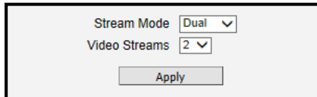
In some types of cameras, other stream mode options are available, such as ePTZ, Fisheye, etc. In this case, select the desired **Stream Mode** and set the **Video Stream** to 1 to ensure that IVS will only use one channel license.
