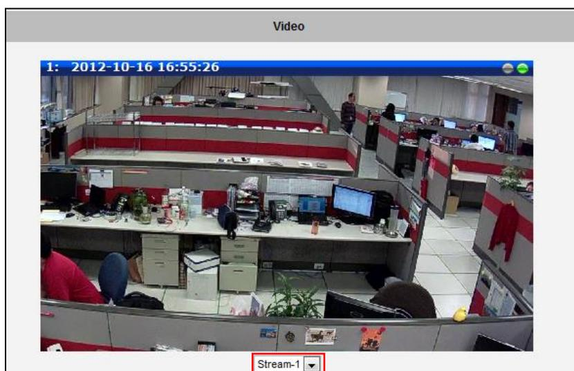
Usually, Stream-1 is configured to be high quality video with maximum resolution and frame rate for recording purposes while Stream-2 is usually a moderate quality stream for live view purposes of the VMS, to reduce VMS computing power during video decoding of multiple channels.
