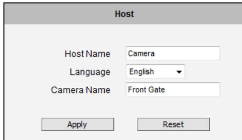
The screenshot shows a web interface titled "Host". It contains three input fields: "Host Name" with the value "Camera", "Language" with a dropdown menu set to "English", and "Camera Name" with the value "Front Gate". At the bottom of the form are two buttons: "Apply" and "Reset".
