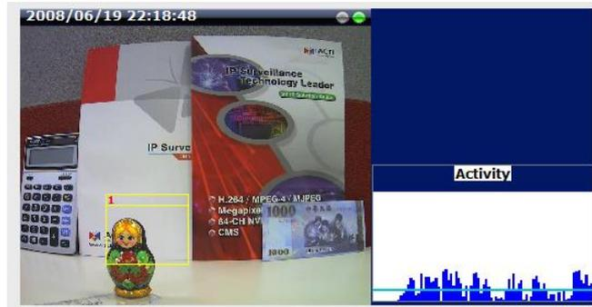
The blue graph on the right side of the image shows how many percent of pixels within the motion detection
