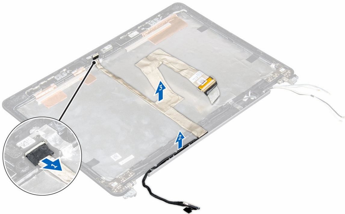
Figure 4. Removing the eDP cable for touch systems
