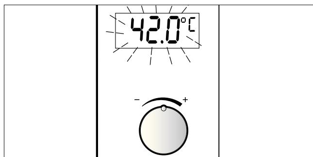
The supply temperature from the domestic system is too high, e.g. water from a solar energy unit.
