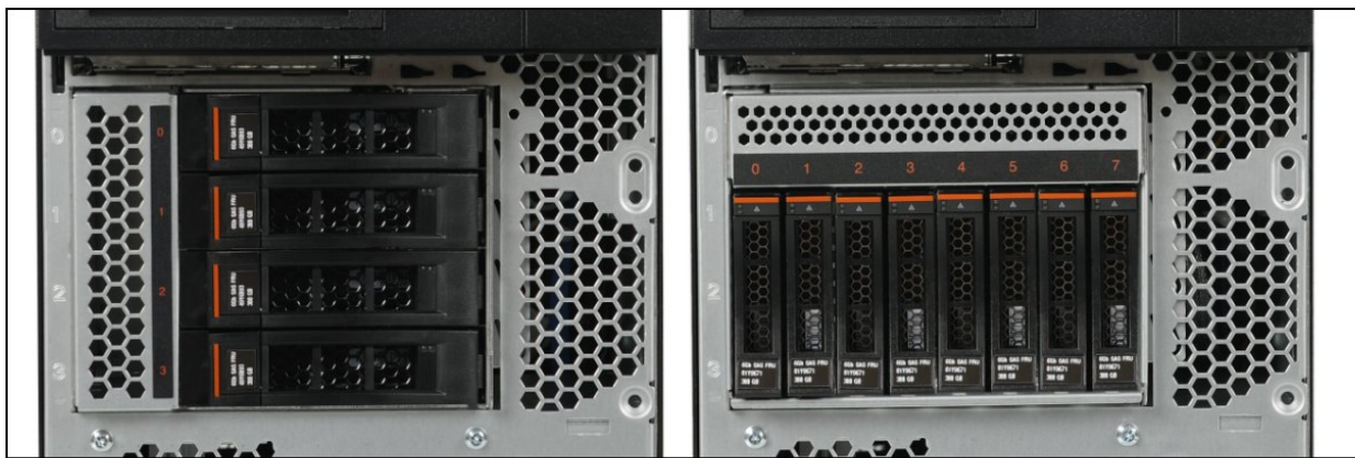
Figure 7. Hot-swap drives that are supported in standard tower models with hot-swap power supplies (front bezel removed) - 4x 3.5-inch (left) or 8x 2.5-inch (right)
