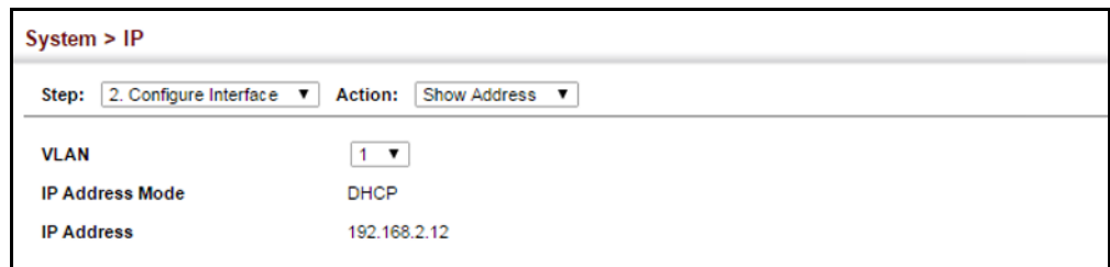
Figure 305: Showing the Configured IPv4 Address for an Interface
