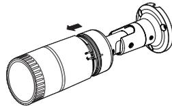
3. Insert a Micro SD card in the arrow direction shown in the figure.
