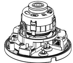
3. Insert the LAN cable into the large hole made by removing the projected part of the rubber plug in step 2 above.
