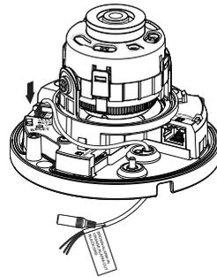
6. Insert the power cable into the small-sized hole through the long, carved groove.
