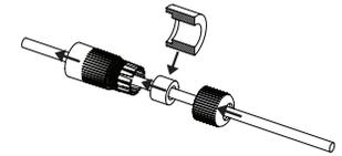
2. Connect the LAN connector (male) to the cable.
