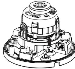
3. Insert the alarm/audio cable through the hole created by removing the rubber cap in No. 2, and connect the cable to the alarm terminal.
