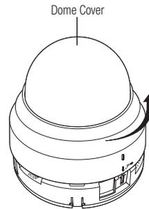
2. Lift up the inner cover to separate it.
