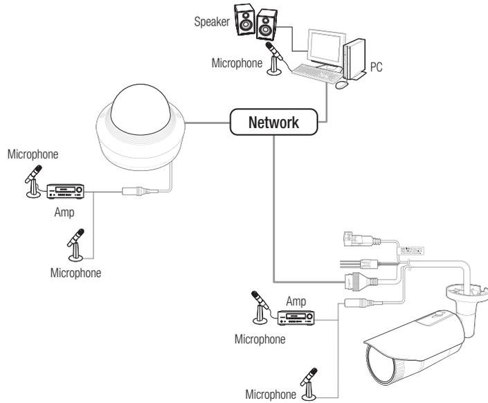
1. Connect the AUDIO IN port of the camera with the microphone or LINE OUT port of the amplifier that the microphone is connected to.
