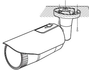
4. Adjust the camera direction using the L wrench provided.
