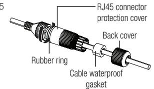
5. Assemble by rotating RJ45 protection cover and back cover clockwise (Follow the arrow). When the back cover is assembled, the cable waterproof gasket is tightly attached to the cable to make it waterproof.
