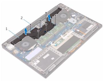
1 heat-sink assembly 2 screws (6)
