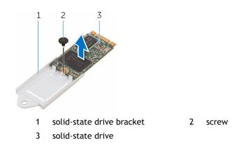
4 Lift the solid-state drive off the solid-state drive bracket.
