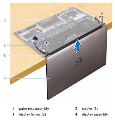
8 Carefully place the display assembly on a clean, flat surface.
