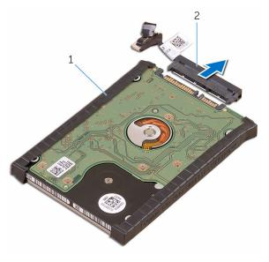
1 hard-drive assembly 2 hard-drive interposer
