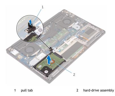
5 Disconnect the hard-drive interposer from the hard-drive assembly.
