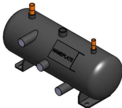
Flooded Receiver, 20L, 219mm diameter, 640mm length, GB with heater
