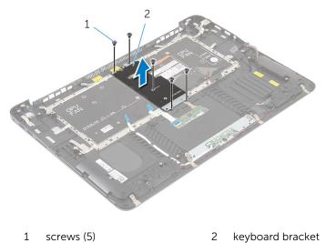
**3** Remove the screws that secure the keyboard to the palm-rest assembly.
