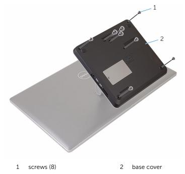
2 Using a plastic scribe, pry up the base cover to release the ports on the system board from the slots on the base cover.
