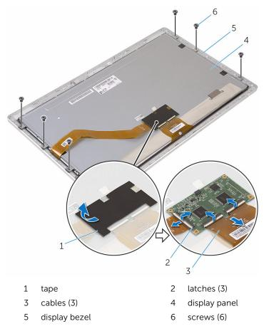
**10** Lift the display-panel assembly off the display bezel and place it on a flat and clean surface.
