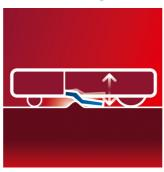
The robot vacuum cleaner comes with a movable nozzle that follows the contours of the floors, carpets, rugs, etc. to ensure accurate cleaning results.
