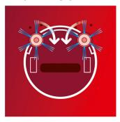
Firstly, the two extra long side brushes swipe dirt and dust into the path of the robot.
