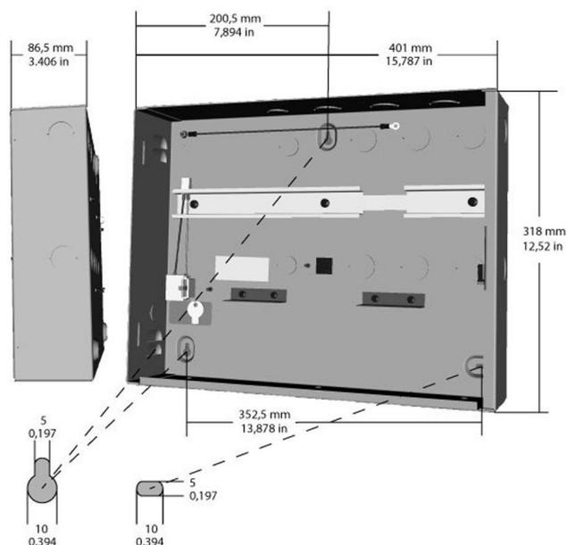
The enclosure is designed for installing an AMC2, a power supply (AMC PBC60) and two batteries.
