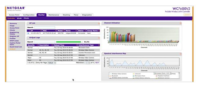
NETGEAR AirQual feature provides at-a-glance view of the RF environment with channel utilization and interference around the WAC740.
