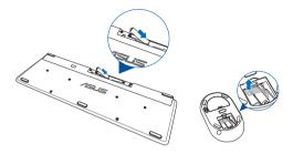
Connect the wireless dongle for keyboard and mouse to the USB 2.0 port to automatically pair both devices to your ASUS All-in-One PC.
