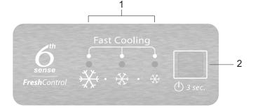
1. Indicator Leds (to display the current temperature setpoint or the Fast Cooling function) 2. On/Stand-By Button / Temperature Button
