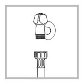
1. Connect the supply pipe by screwing it to a cold water tap using a ¾ gas threaded connection (see figure). Before performing the connection, allow the water to run freely until it is perfectly clear.
