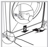
3. remove the cover panel on the lower front part of the washer-dryer (see figure).
