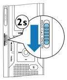
2 To power off, pull down the power switch on the side of the device again and hold for about two seconds.
