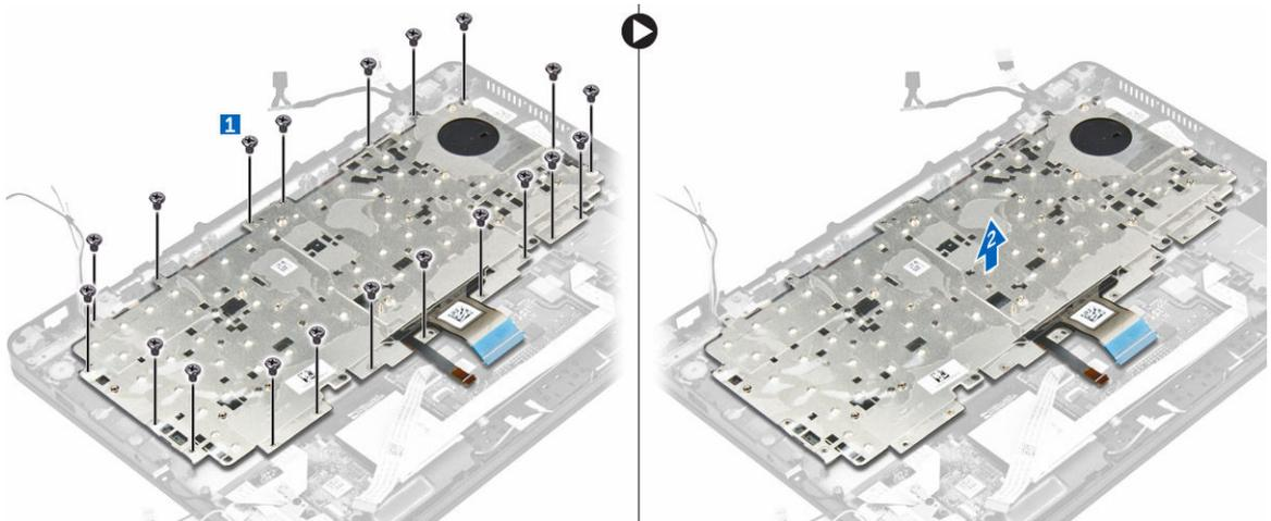
5. Remove the screws that secure the keyboard [1] to the computer and lift the keyboard from the computer [2].
