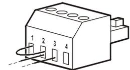
**Note:** Pin 1 is the power source for the EPO circuit, it provides a few milliamperes of 24 V power.
