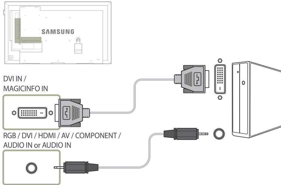
— You can use the DVI port on the product as an HDMI port by using a DVI-HDMI adapter.
