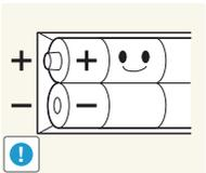
Use only the specified standardized batteries, and do not use a new battery and a used battery at the same time.
