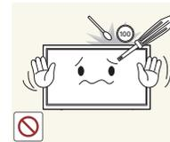
Do not insert metallic objects (chopsticks, coins, hairpins, etc) or objects that burn easily (paper, matches, etc) into the product (via the vent or input/output ports, etc).
