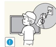
Before moving the product, turn off the power switch and disconnect the power cord, antenna cable and all other connected cables.
