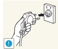
Connect the power plug to a grounded power socket (type 1 insulated devices only).
